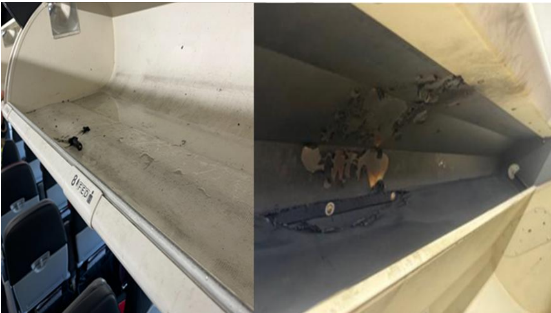
Figure 7: Overhead locker above row 7DEF where the smoke and flames were observed (left) and area behind the overhead locker showing fire damage (right)
