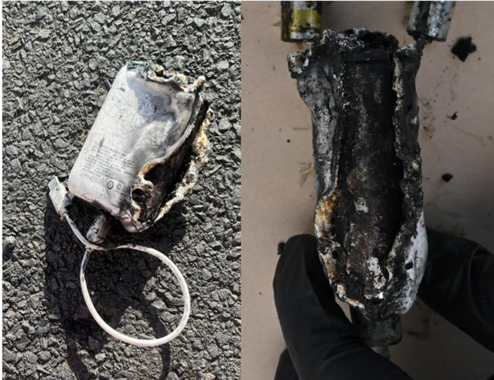
Figure 6: Power bank showing damage from the back (left) and side view (right)
