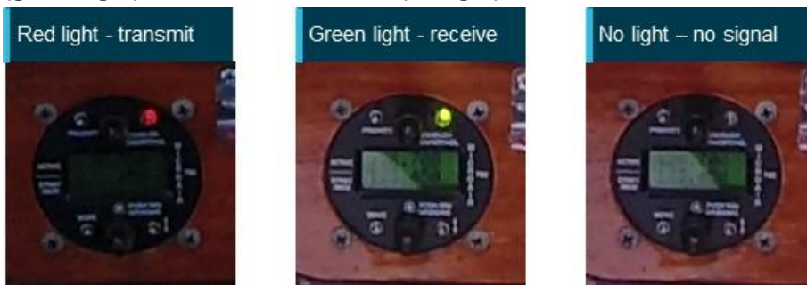
Figure A1: Screen captures of the radio fitted to 19-4079 during send (red light), receive (green light) and no transmissions (no light)
