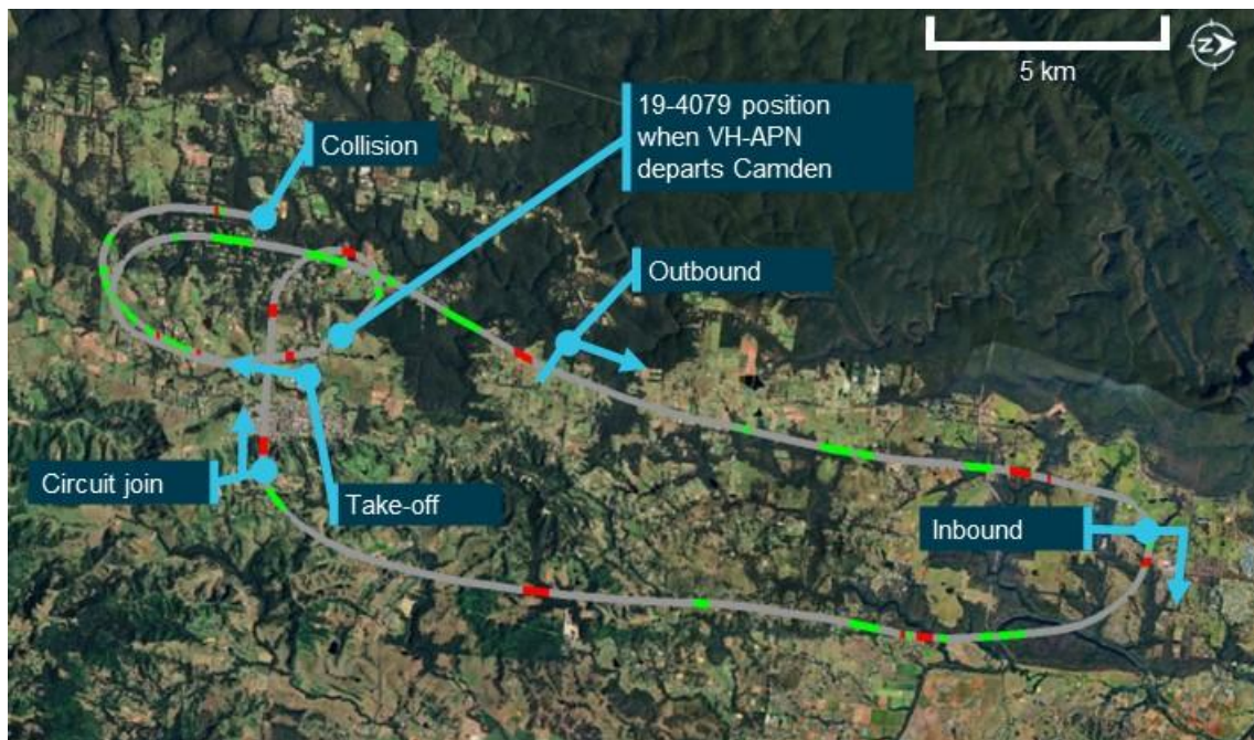
Figure 10: Flight track showing the position of 19-4079 when no transmission was detected (grey lines), and when radio calls were transmitted (red lines) and received (green lines) by 19-4079 during the accident flight
