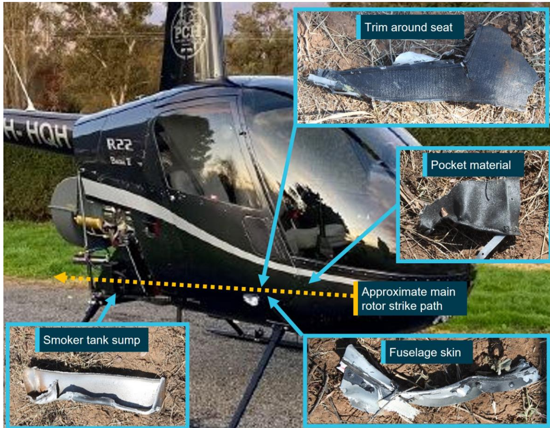
Figure 9: VH-HQH (pre-accident) showing approximate location of rotor strike and first items in debris field
