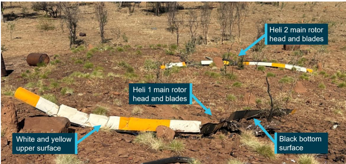
Figure 5: High visibility main rotor blades
