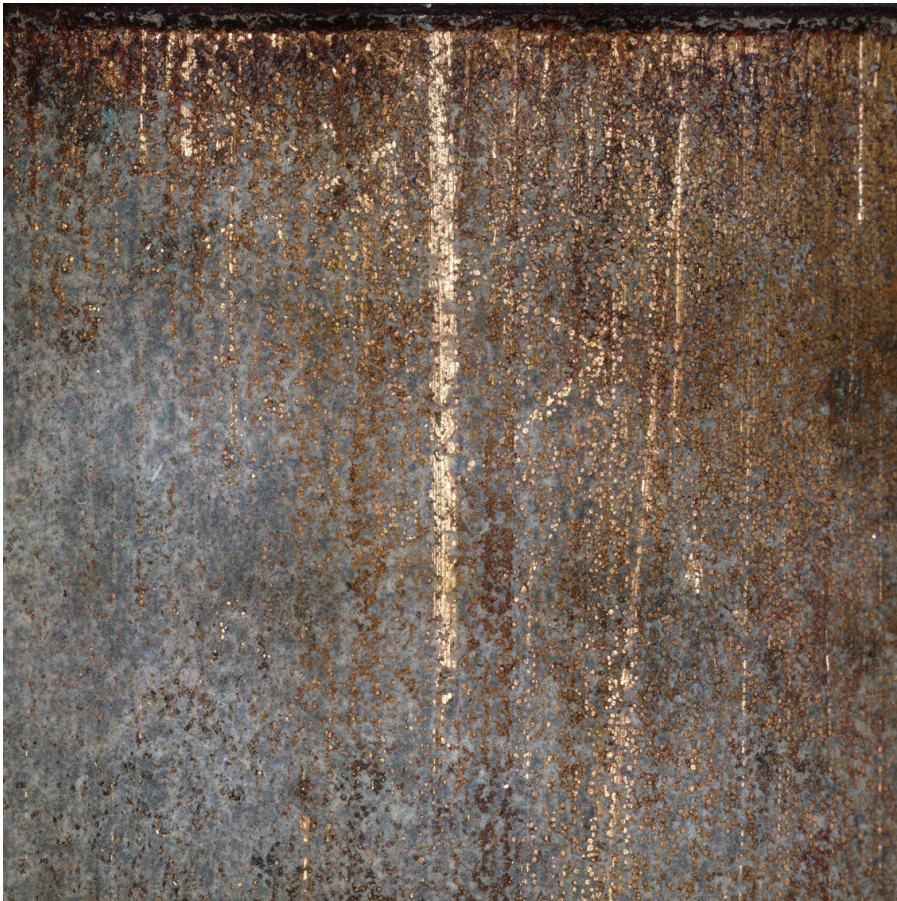
Figure 11: Right carriage bushing surface showing Teflon/lead layer (grey), exposed bronze layer (copper) and some evidence of scoring (bright lines)
