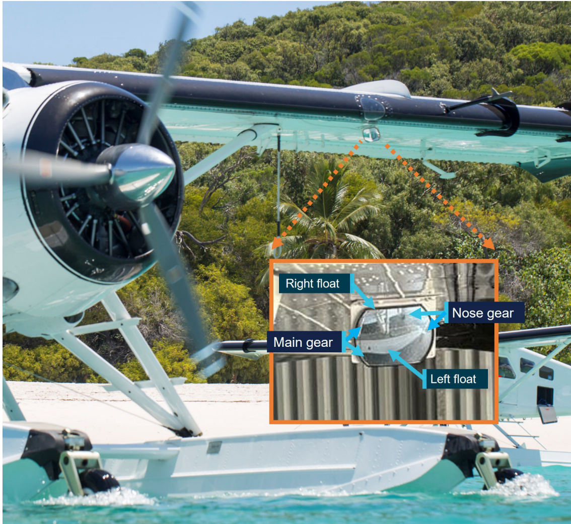
Figure 7: Left wing mirror location, with representation of extended gear visible view
