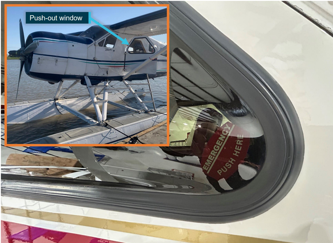
Figure 12: Example of main cabin door push-out window
