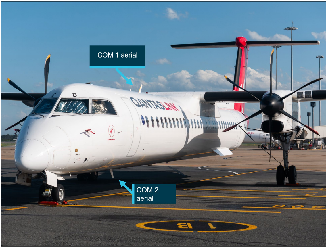
Figure 3: Dash 8 with annotations of VHF antenna locations on airframe
