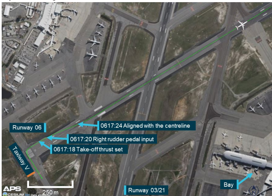
Figure 1: Overhead of Perth Airport and showing the aircraft's line up on runway 06 with key events during the take-off for incident 1
