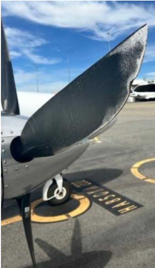
Figure 4: Damage to propeller blade on right engine
