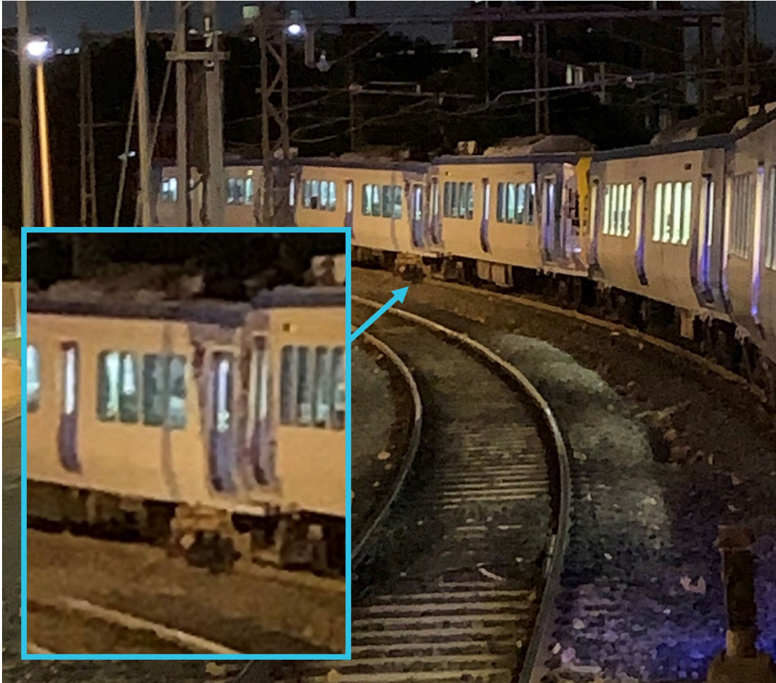
Figure 5: View of derailment from the front of the train
