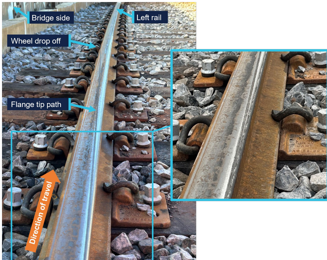
The figure shows the flange climb mark made by the tip of wheel flange looking in the train's direction of travel. The inset shows additional detail along the rail gauge corner. Source: OCI
