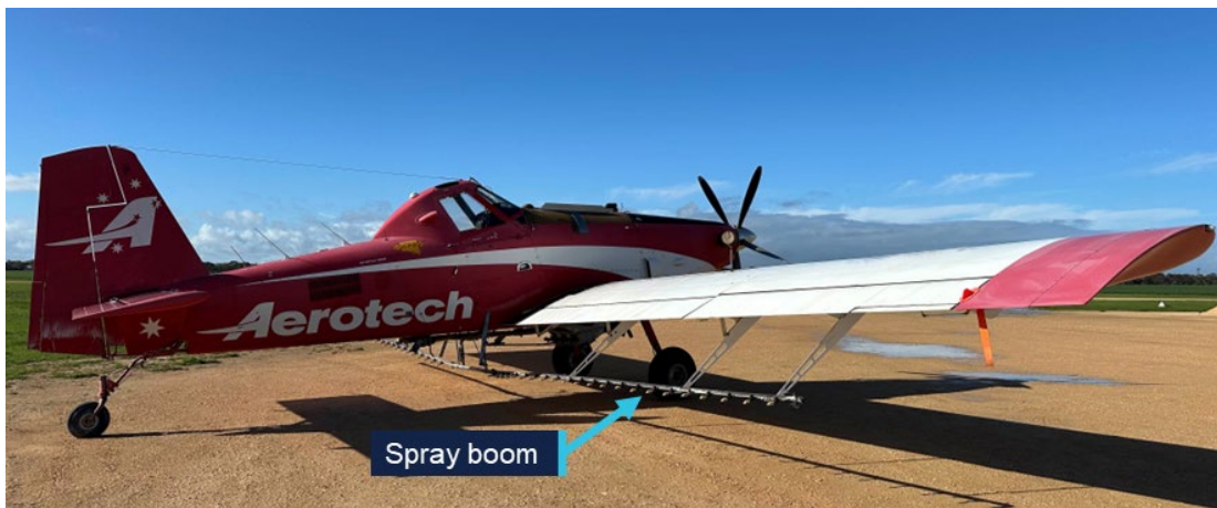
Figure 4: Exemplar AT-802 showing spray boom installation
