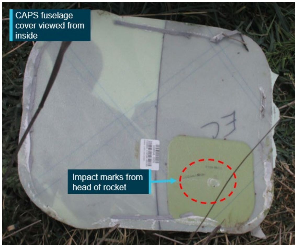
Figure 17: CAPS external cover showing internal impact mark
