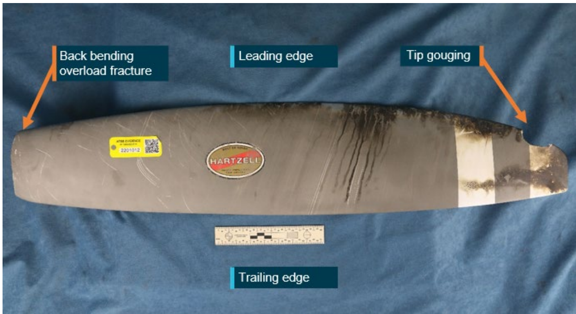
Figure 19: Blade C as recovered from the accident site
