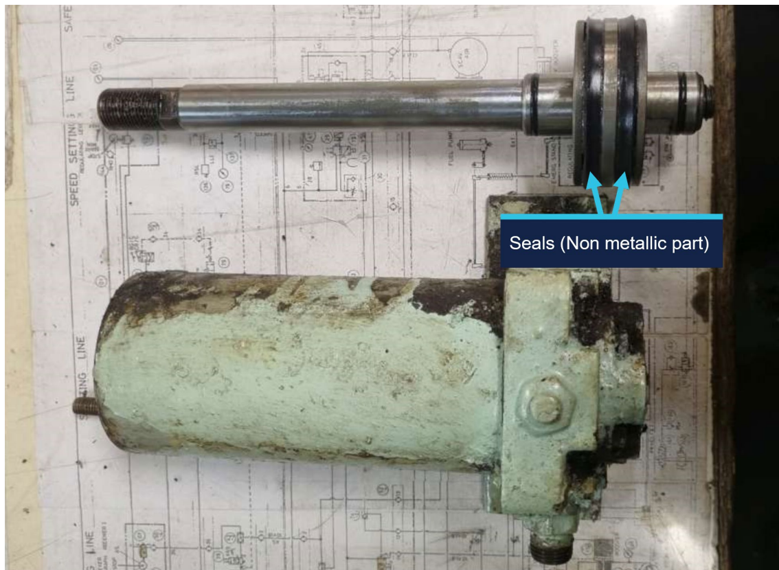
Figure 5: Main air distributor reversing cylinder/servo piston with new seals
