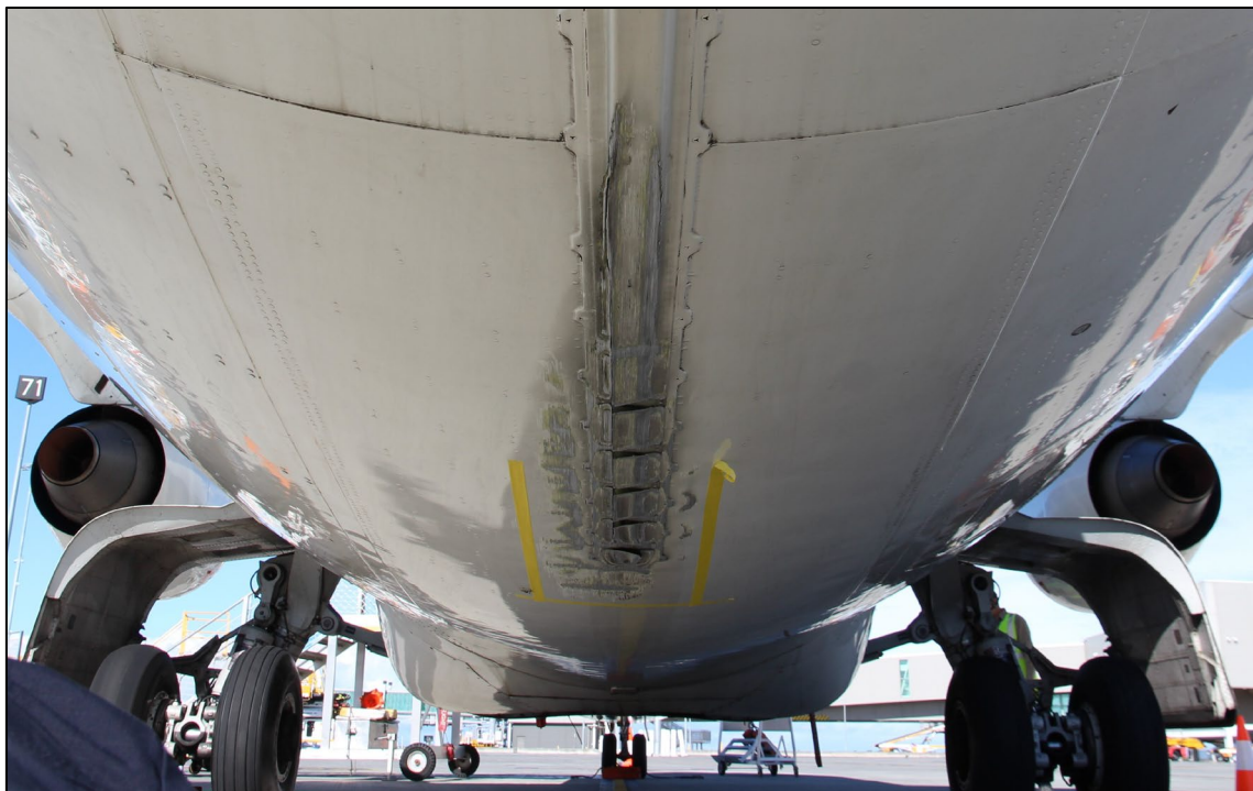
Figure 3: VH-SAJ damage to tail strike indicator and surrounding panels
