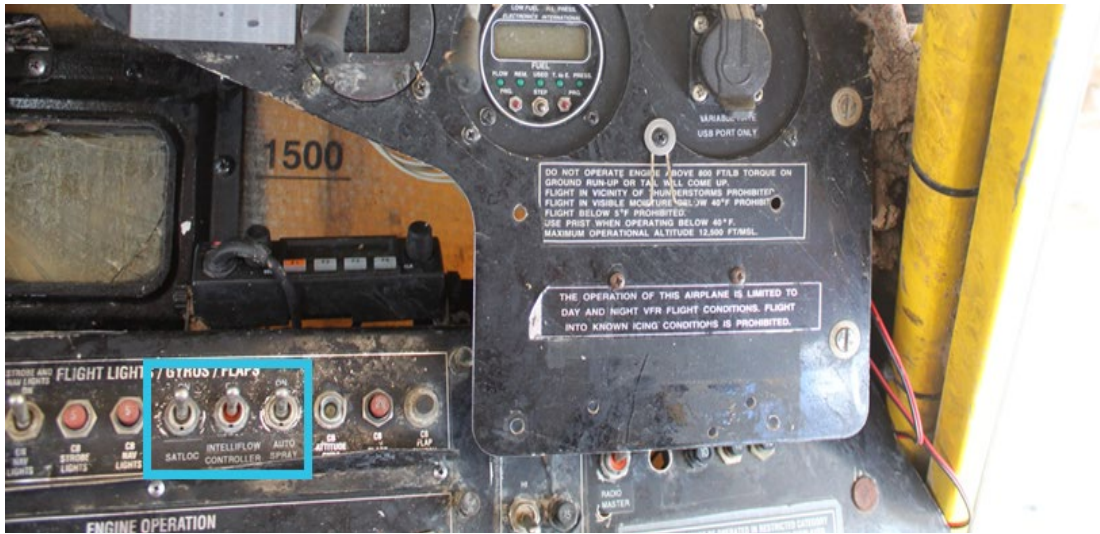
Figure 2: Switches (in box) used for spraying in VH-AQW
