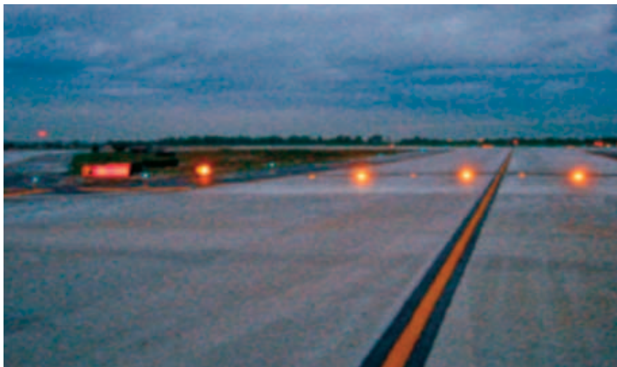
Runway holding point as viewed from a taxiway centreline. This holding point has both above ground and in-pavement runway guard lights.
