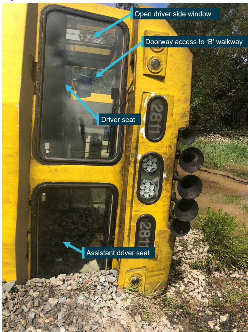
Figure 17: Derailed lead locomotive 2811 no 2 end cab
