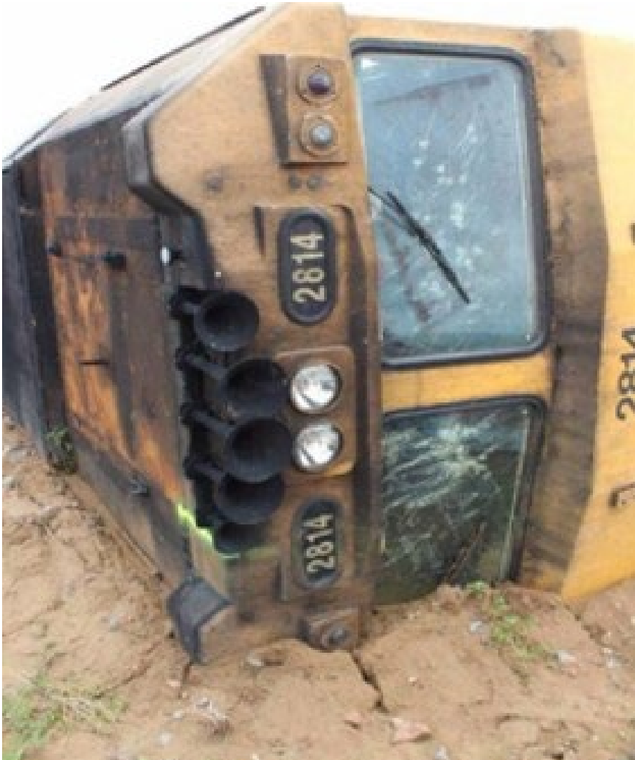
Figure 15: Excerpt from Aurizon guideline showing windscreen damage from repeated strikes from the window hammer
