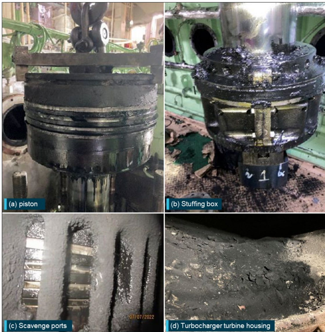
Figure 11: Condition of some engine components
