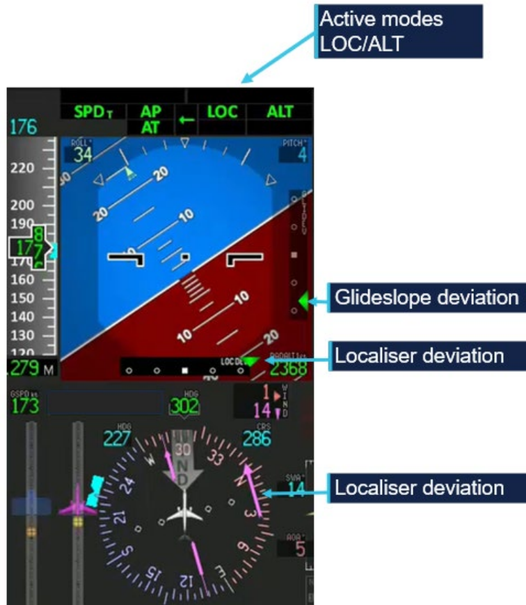
Figure 6: Primary flight display at 1636:22 showing full-scale localiser deviation (localiser right of the aircraft) and nearly 2 dots glideslope deviation (glideslope below the aircraft)
