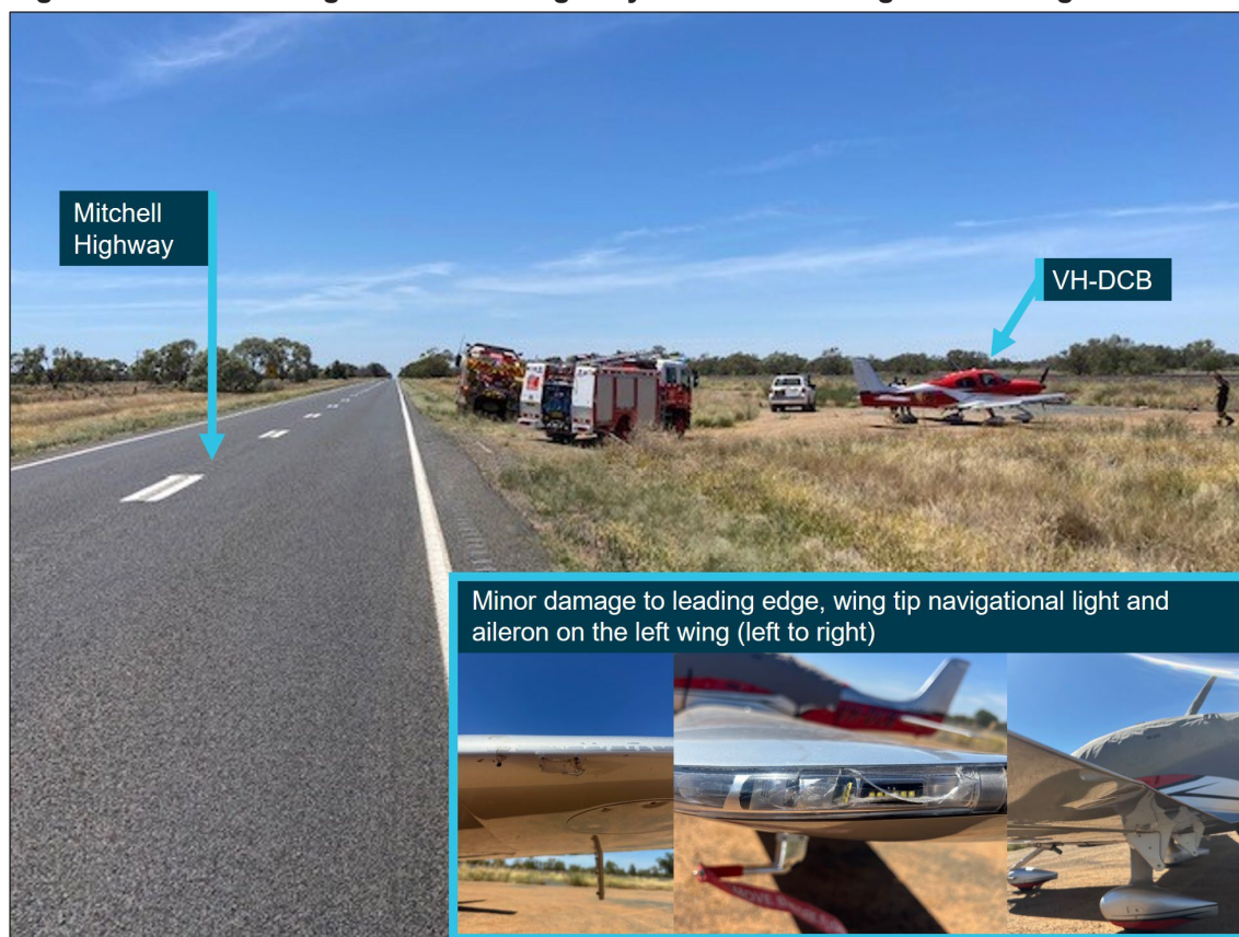
Figure 2: VH-DCB alongside Mitchell Highway and minor damage to left wing
