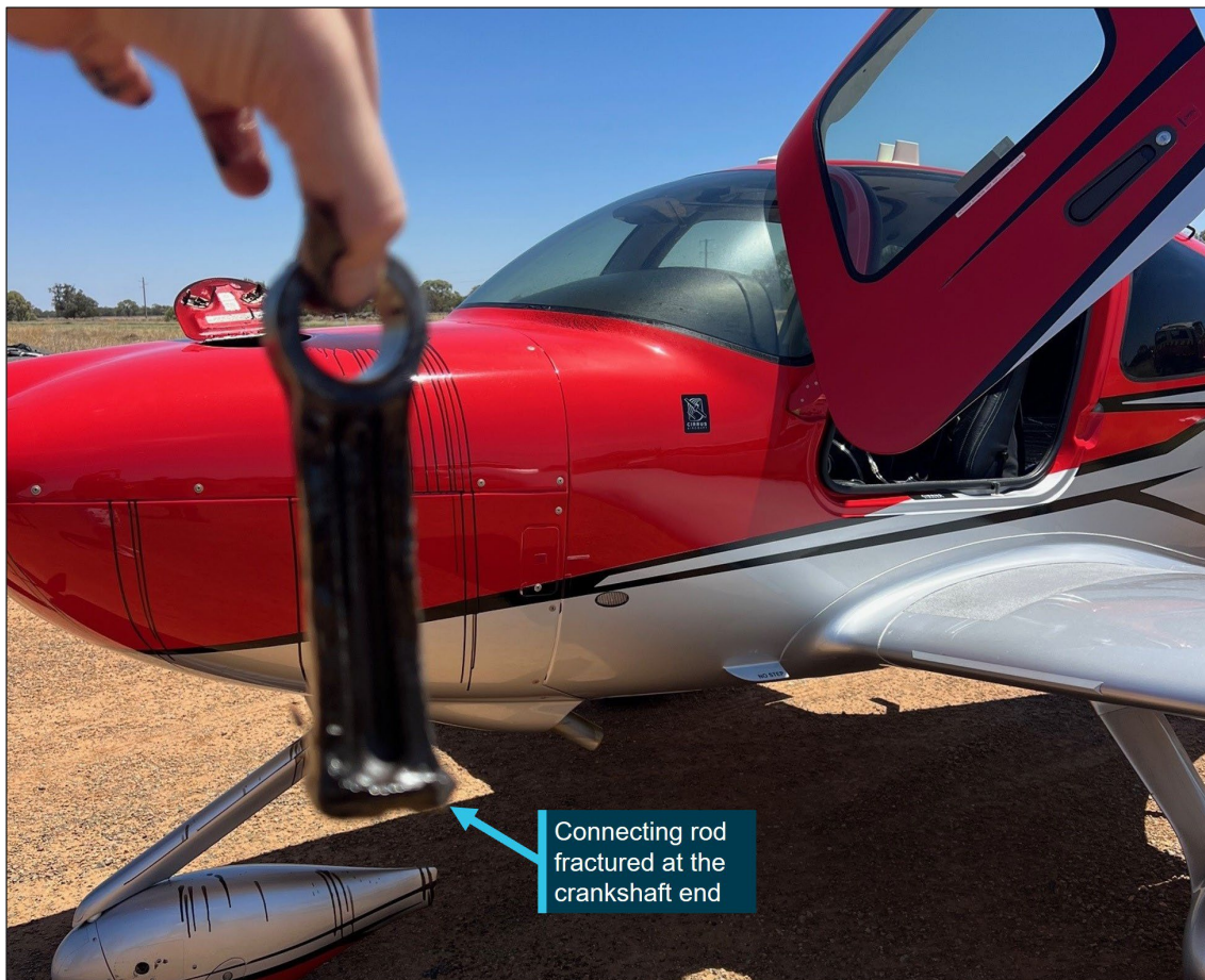
Figure 4: Fractured connecting rod recovered from VH-DCB
