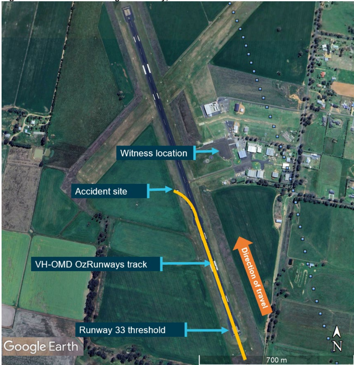
Figure 3: VH-OMD track along the runway, accident site and witness location
