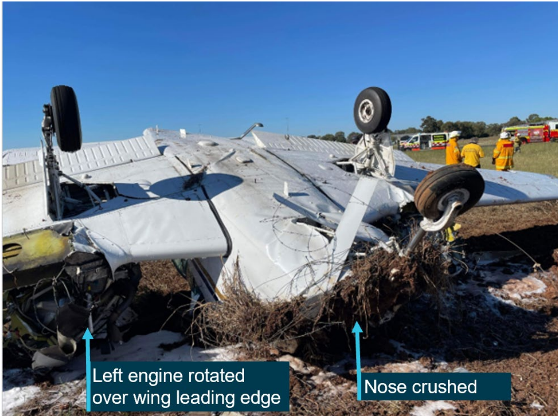
Figure 7: Impact damage to VH-OMD
