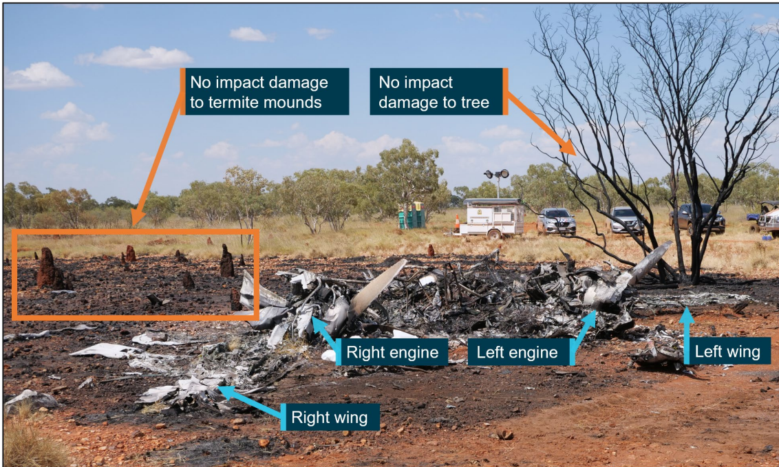
The surrounding landscape features (termite mounds and a tree) remained upright and were not disturbed from the impact. Source: ATSB
