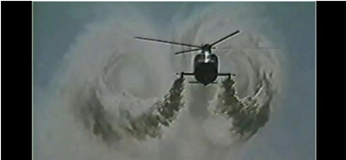
Figure 3: Rotor wake vortices visualised with smoke generators
