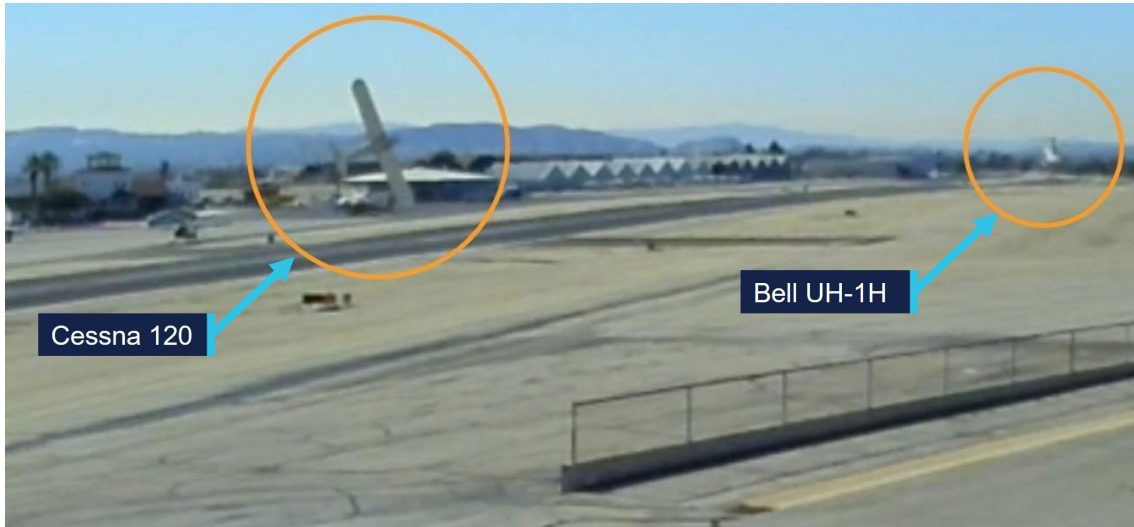
Figure 5: Loss of control accident from rotor wake
