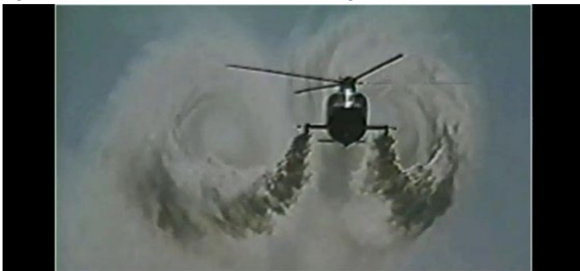
Figure 3: Rotor wake vortices visualised with smoke generators
