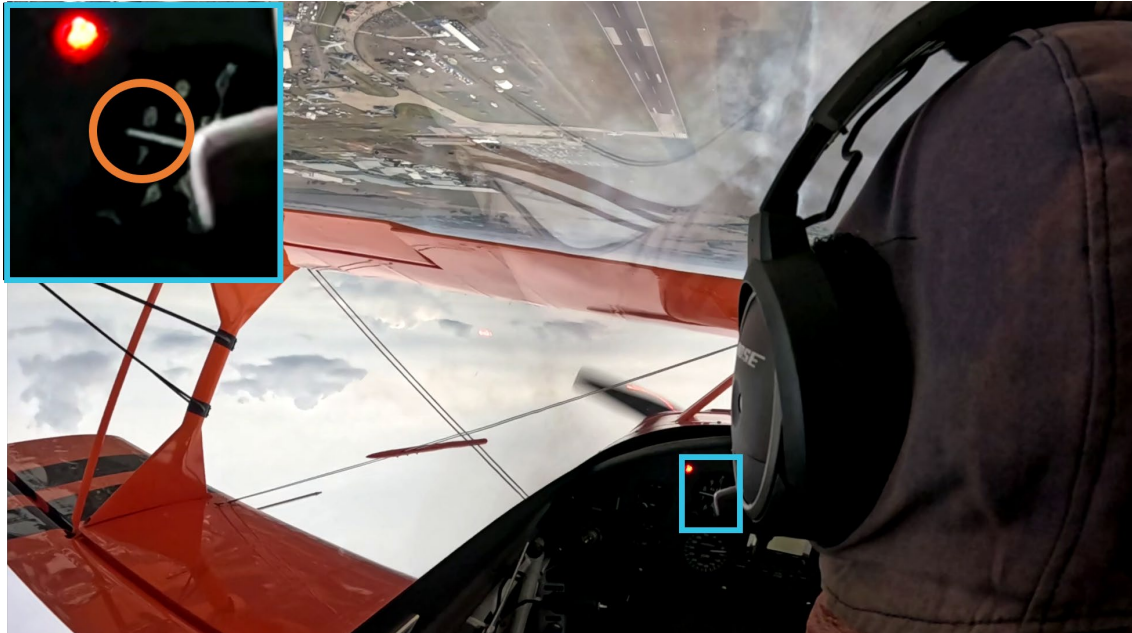
Figure 5: Still image from the accident flight recording showing the altimeter just prior to the first snap roll during the triple avalanche manoeuvre
