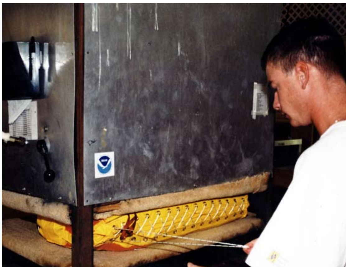
A life raft and its survival equipment pack are laced tightly during packaging under pressure.
