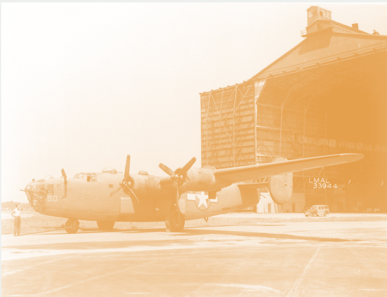
Known as a ‘bad ditcher,’ the Consolidated B-24 Liberator bomber did not have safety belts for all 10 crewmembers, and a bulkhead tended to collapse on impact.
