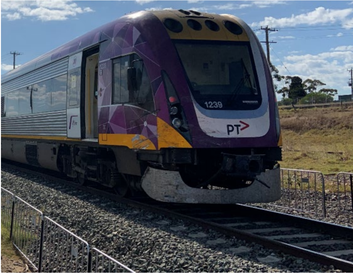
Figure 9: Damage to the front of train 7727
