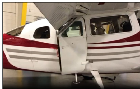
Hinged forward cargo door. Source: Coast Dog Aviation
