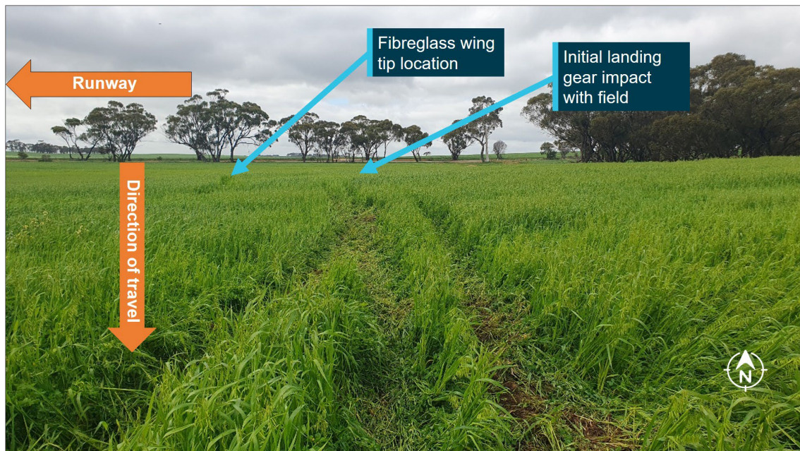
Figure 3: Aircraft landing gear marks in field adjacent to the runway
