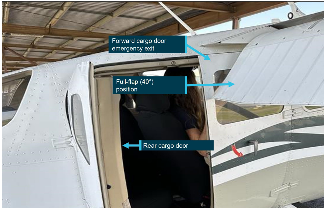
Figure 6: Cessna 206H showing extended flap blocking forward cargo door
