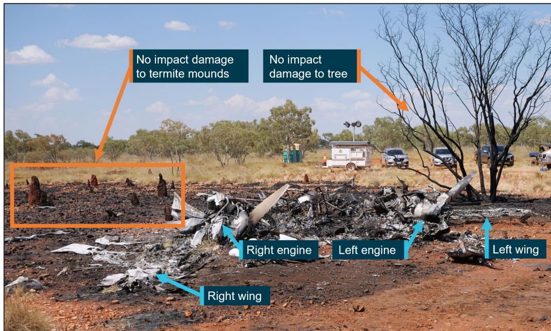
Figure 13: Heavily disrupted and burnt remnants of the wreckage at the accident site
