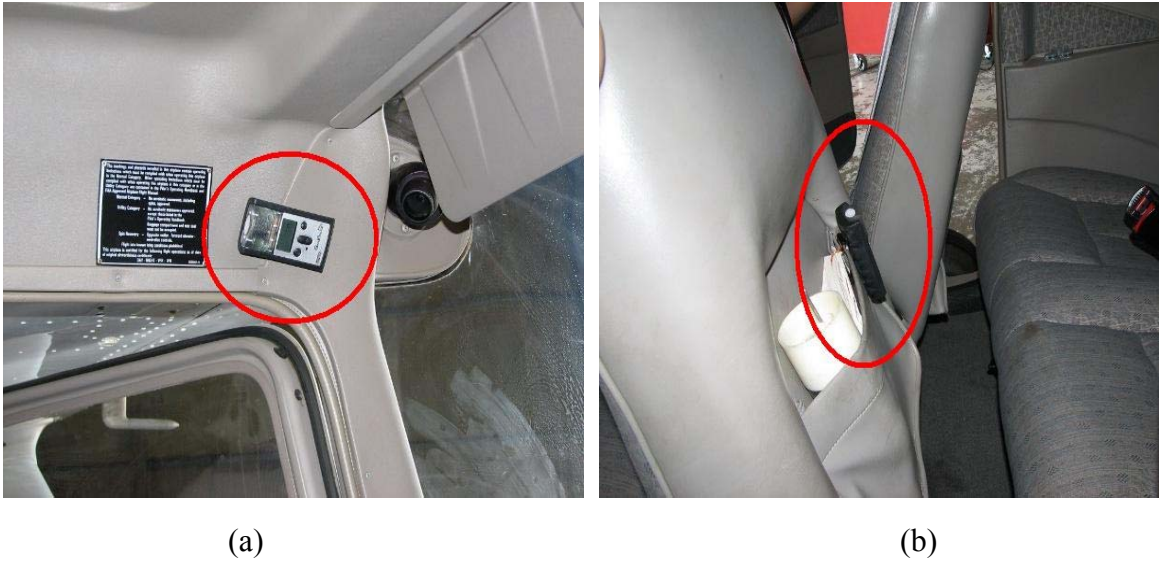
Figure B-3. Carbon Monoxide Detectors Located (a) Near the Pilot-Side Visor and (b) the Back-Seat Area With Suspender Clips
