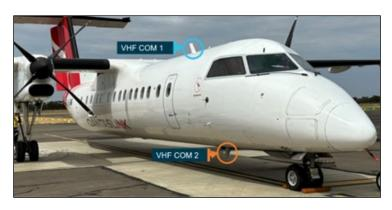
Dash 8 300 aircraft while using VHF COM 2 for ground-based very high frequency (VHF) communications.
