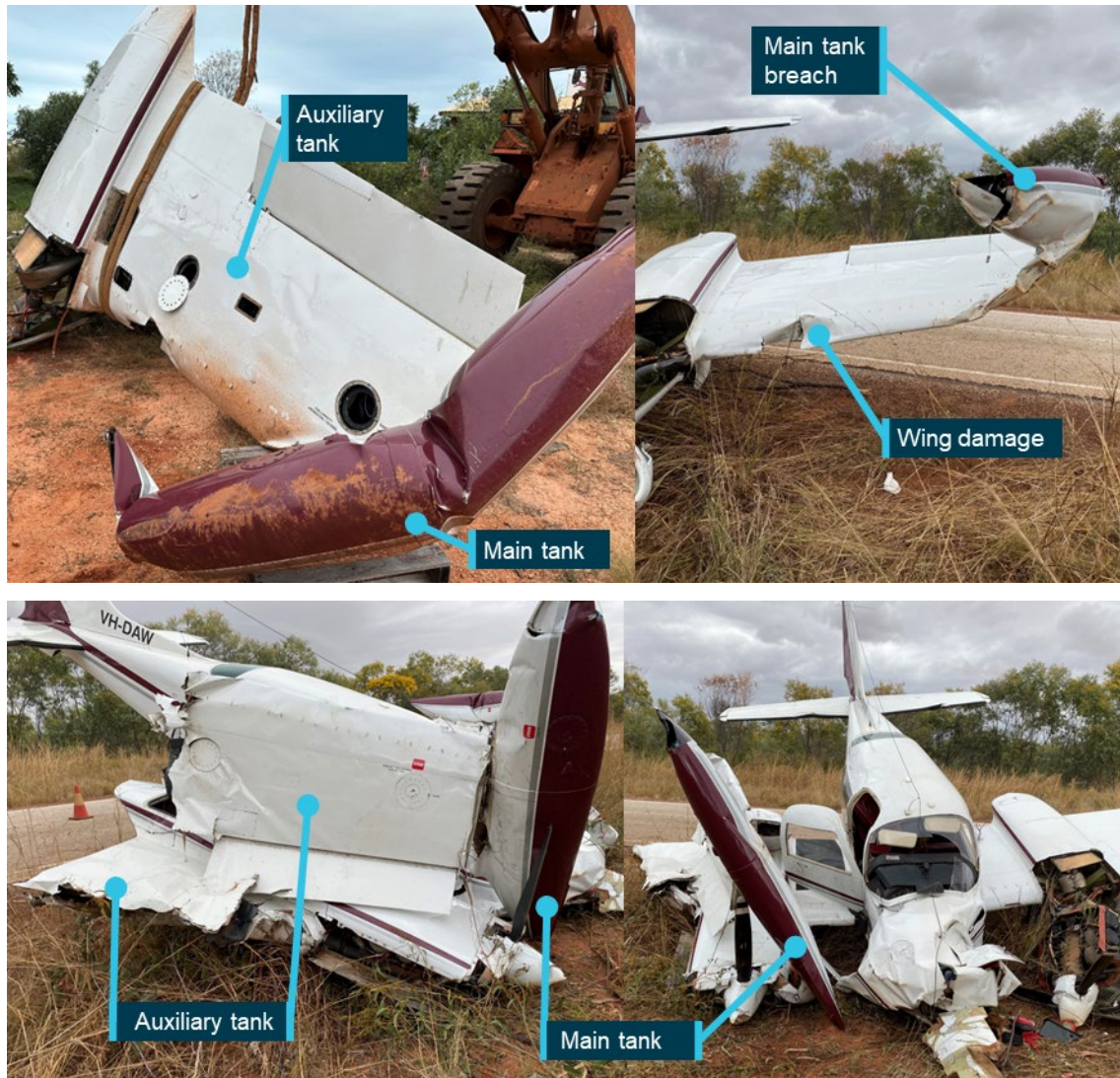
Figure 5: Left and right wing damage
