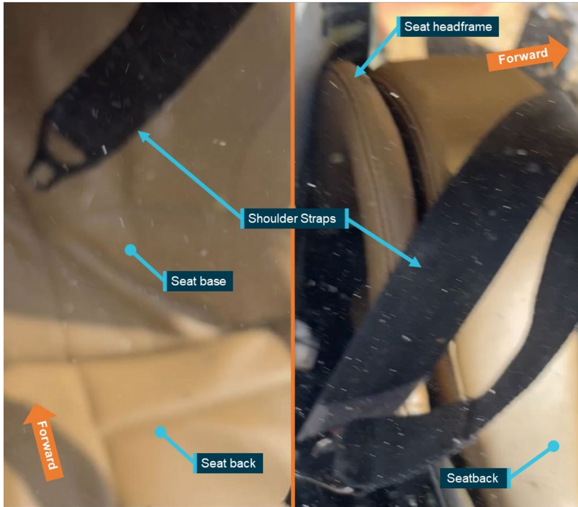
Figure B1486: Front right seat shoulder harness disconnected during rollover
