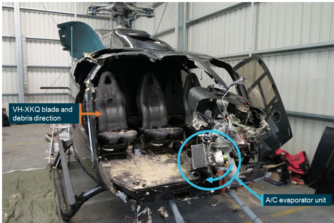
Figure B5: VH-XH9 air-conditioning cockpit evaporator unit distorted in the direction of VH-XKQ's travel
