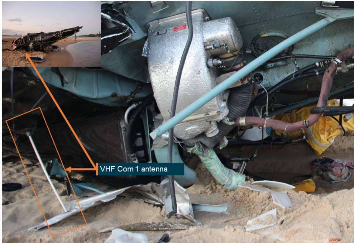
Figure 44: The VHF Com 1 antenna (main) from XKQ at the accident site (inset)
