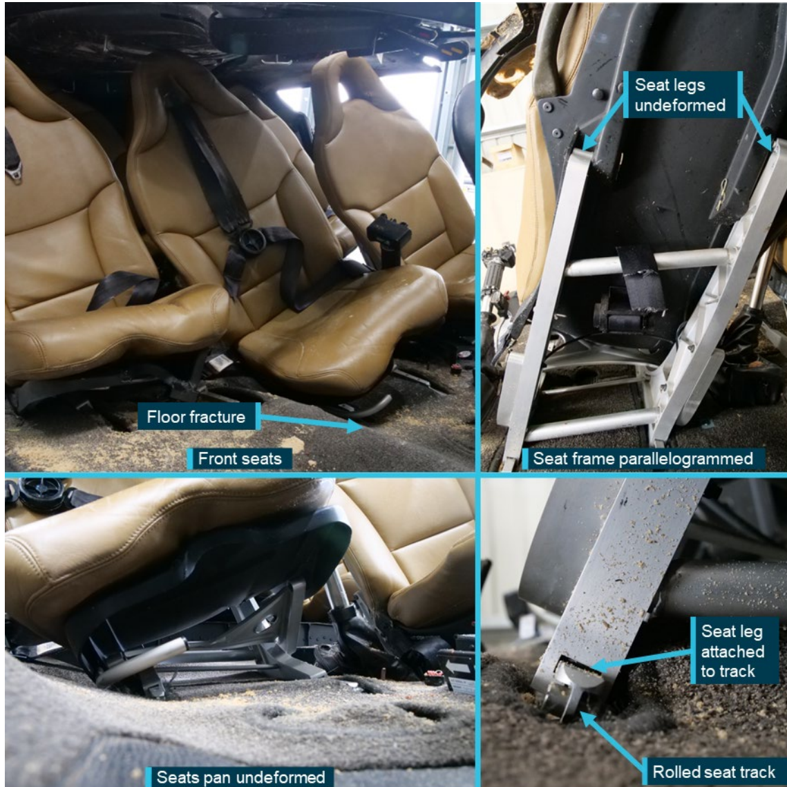
Figure B12: Composite picture of typical seat damage
