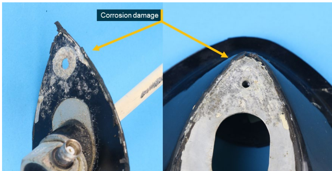
Figure A3: Corrosion damage to the fix hole surfaces surrounding where the antenna mounting plate (left) was attached to the blister panel (right)
