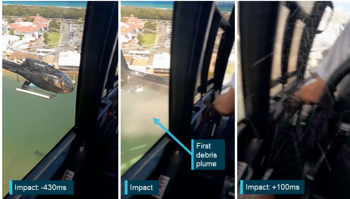
Figure B2: VH-XKQ initial main rotor blade strikes to VH-XH9
