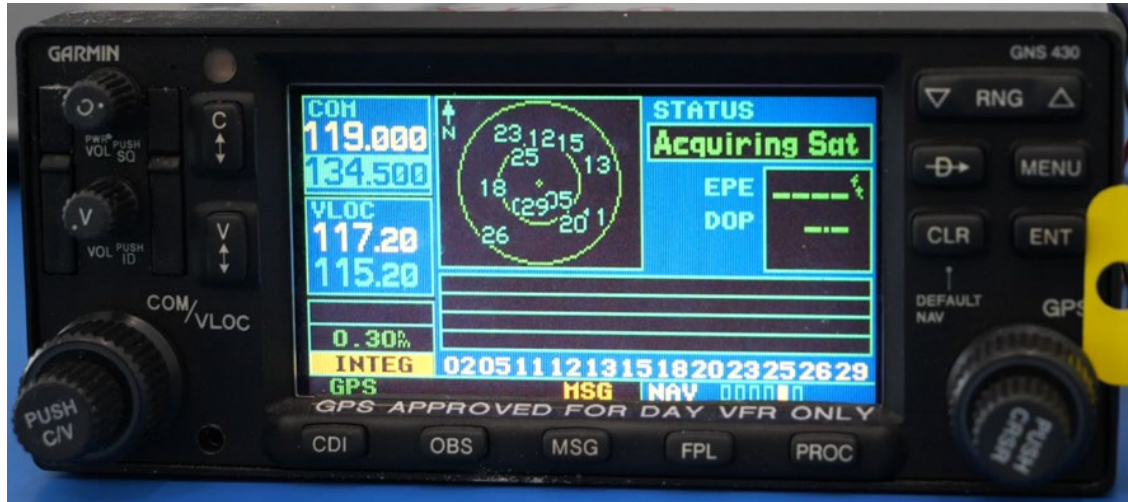
Figure 21: Garmin GNS430 (Com 1) from VH-XKQ – indication on power up after self-test
