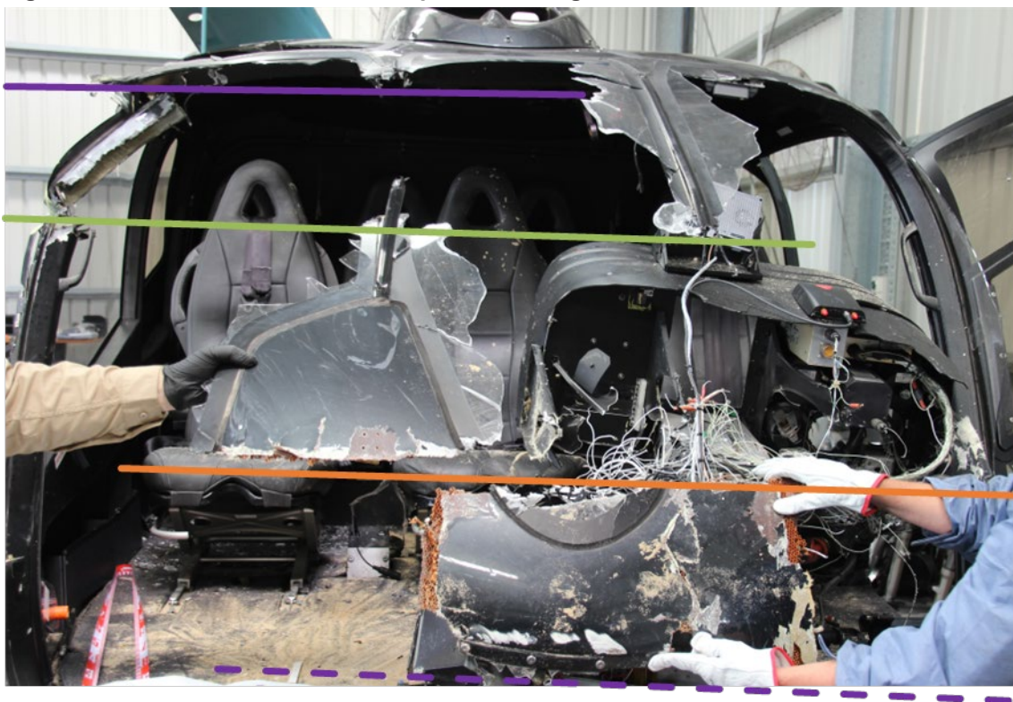
Figure B3: VH-XKQ main rotor blade passes through cabin of VH-XH9
