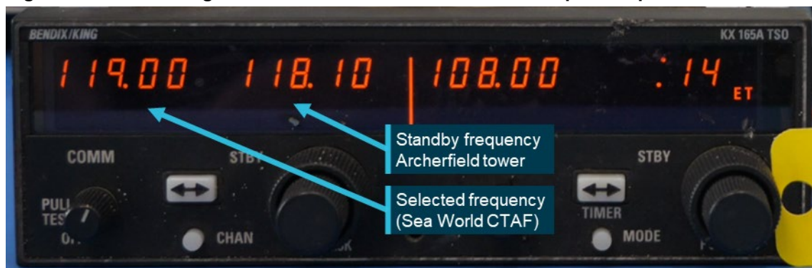
Figure 20: Bendix King KX-165A from VH-XH9 – indication on power up
