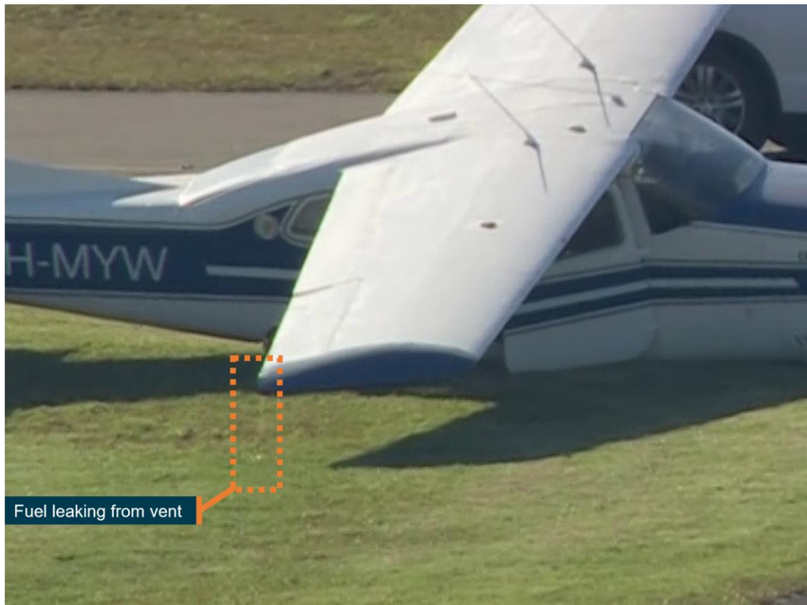
Figure 5: Fuel leak from right tank vent
