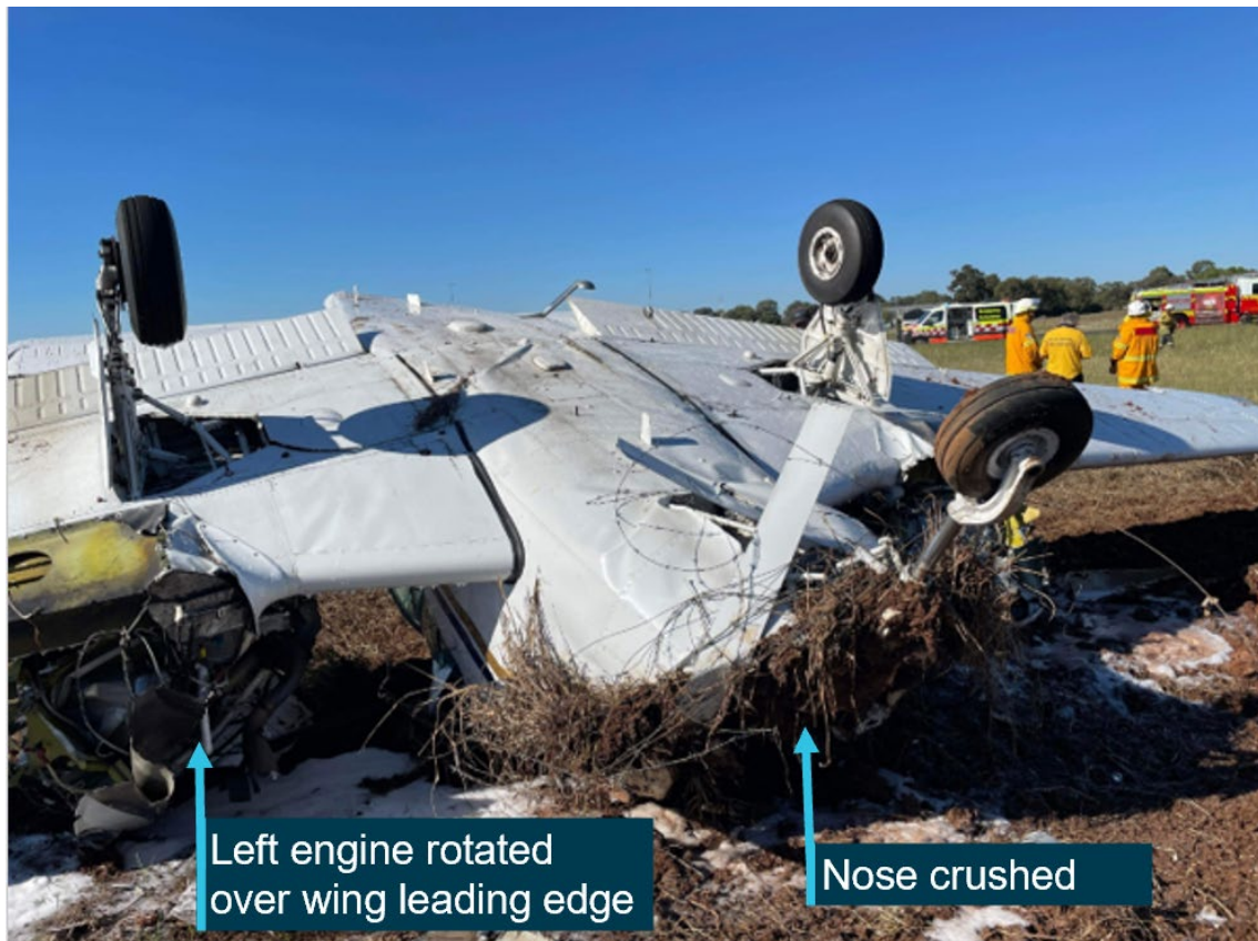
Figure 7: Impact damage to VH-OMD
