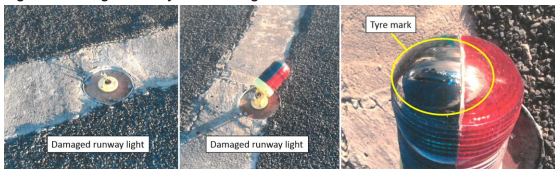
Figure 2: Damaged runway threshold lights
