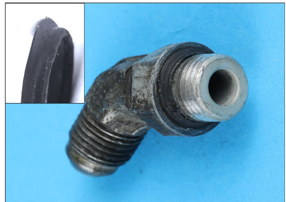
Age-affected O-ring seal of fluid carrying fitting with inset image displaying permanent deformation of the seal (Source: ATSB)
