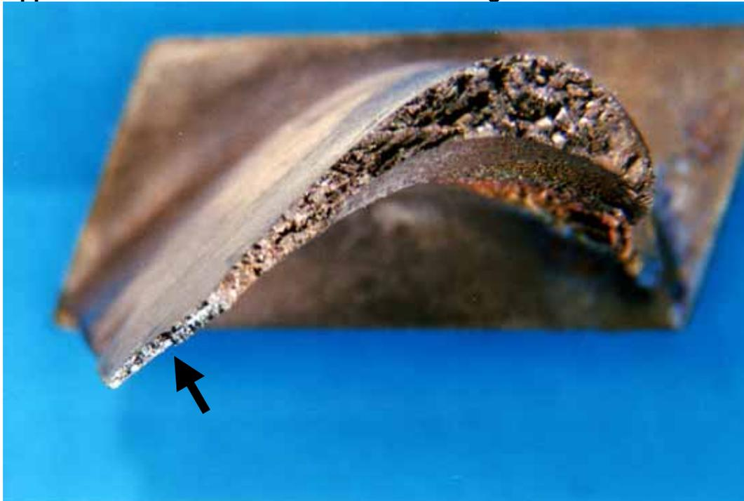
Region of crack growth with faceted 'faceted' features, arrowed (delineated by the blue heat tinting)
