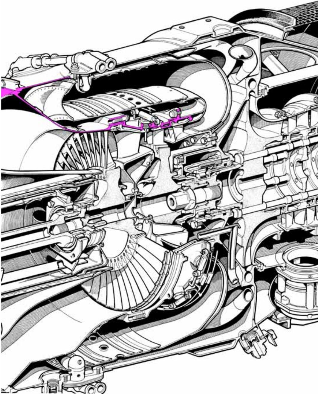
Cutaway diagram of a PW&C PT6-27 engine
