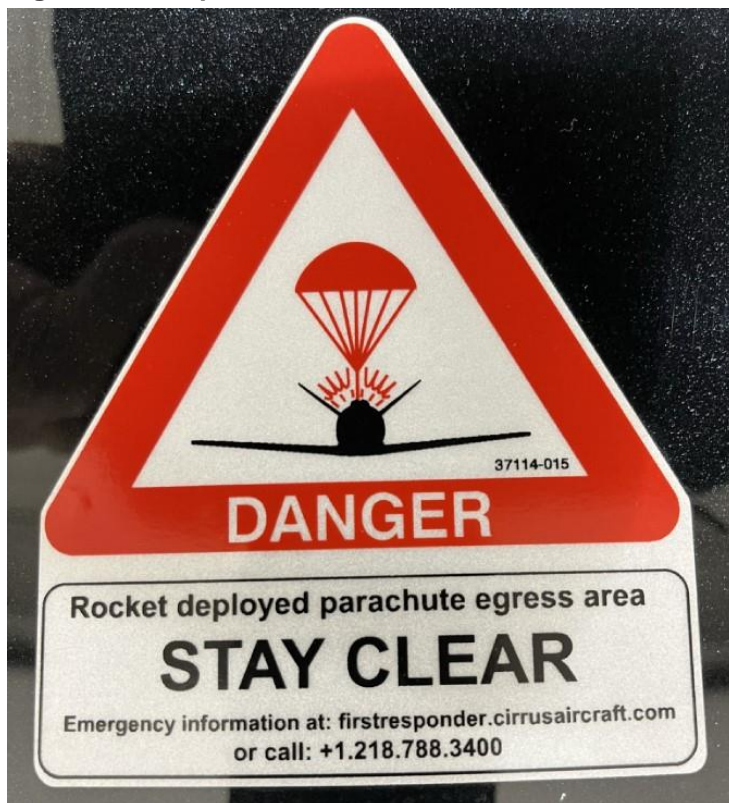
Figure 8: Example of an ASTM Standard CAPS Placard used on the SF50 Vision Jet
