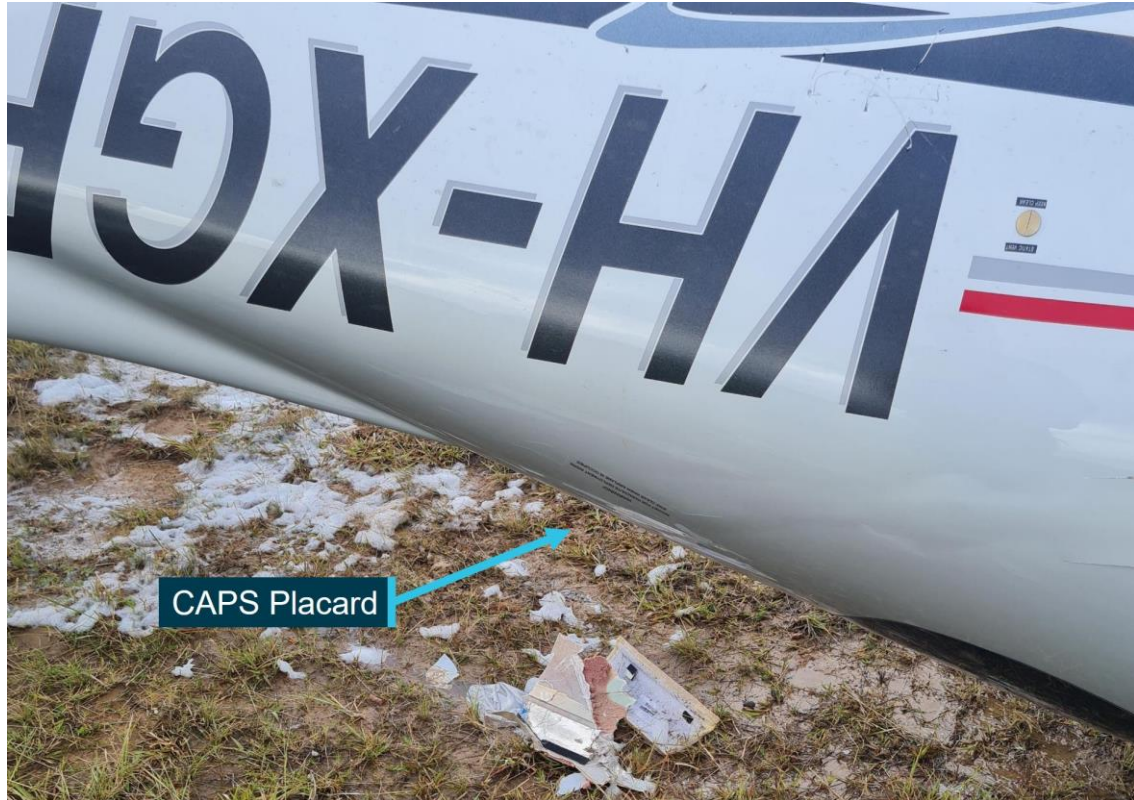
Figure 7: Wreckage (inverted) at accident site showing CAPS warning placard on left rear fuselage
