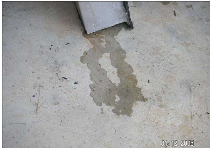
Figure 16: Water leaking from the fuel tank during testing
