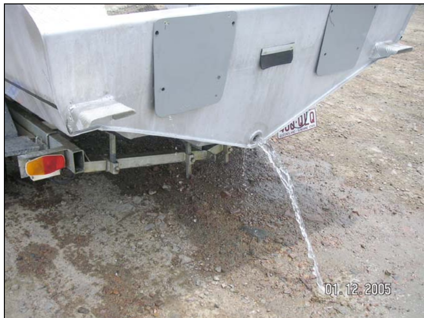
Figure 24: Water draining from void
