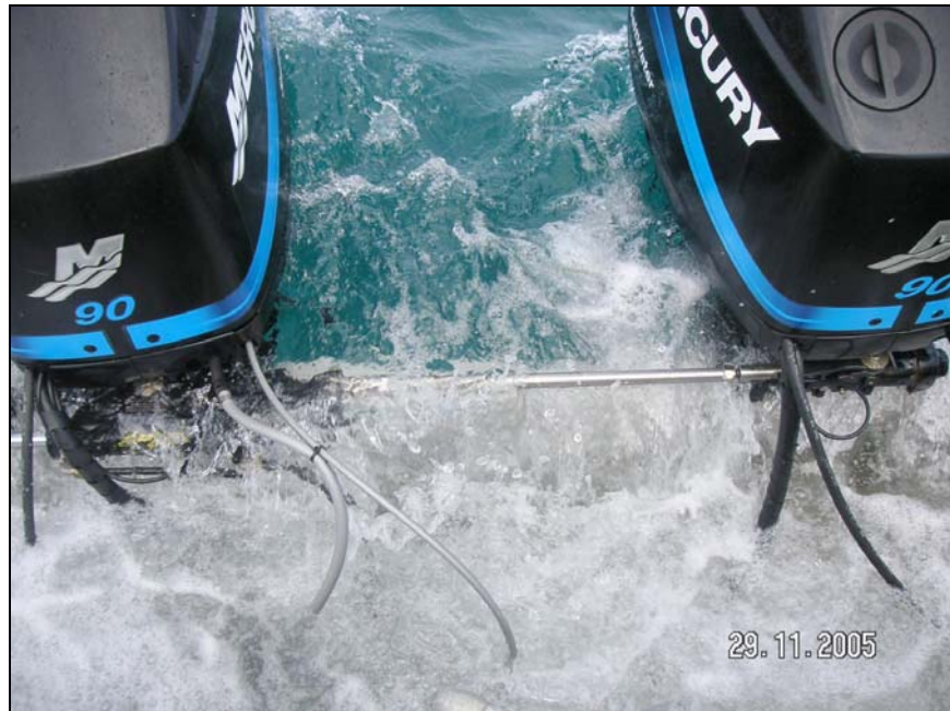
Figure 4: Stern motor well flooding
