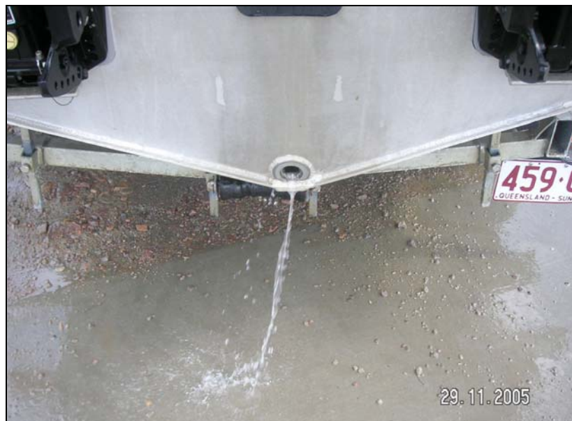
Figure 7: Water draining from the void
