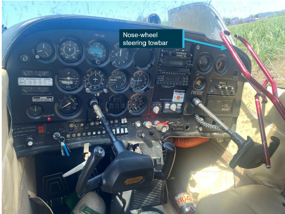
Figure 4: Nose-wheel steering towbar unrestrained in the cockpit
