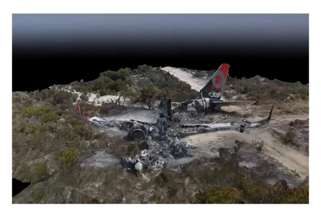
ATSB produced a 3D model of the 737 large air tanker accident site using the capability of its RPAS
