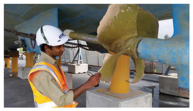
An ATSB investigator examines a vessel's damaged propeller
