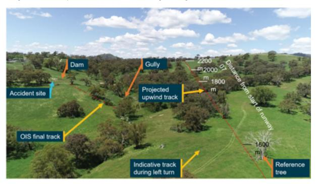
Figure 3: Image looking uphill at a similar height and position to VH-OIS prior to the accident
