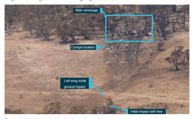
Figure 4: Accident site overview showing the wreckage trail
