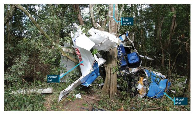
Figure 2: The main wreckage of VH-CYO at the base of a large tree that was struck
