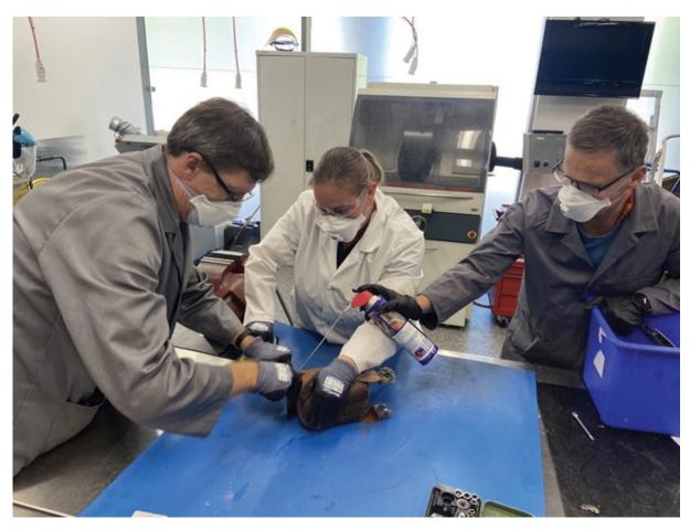
ATSB investigators examining fire damaged recorder from the Boeing 737 large air tanker accident
