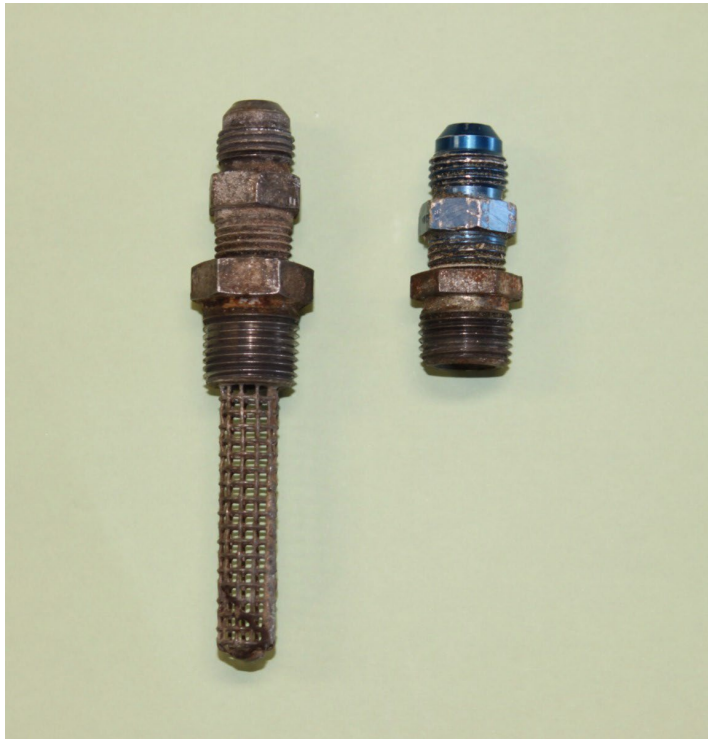
Figure 3: VH-FEY Fuel tank outlet fittings - left with finger strainer and right without finger strainer
