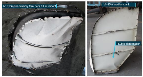
Figure 20: An exemplar auxiliary tank known to be nearly full at impact and VH-IDW's
