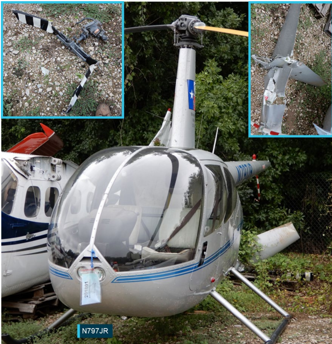
Figure 24: N797JR post in-flight break-up
