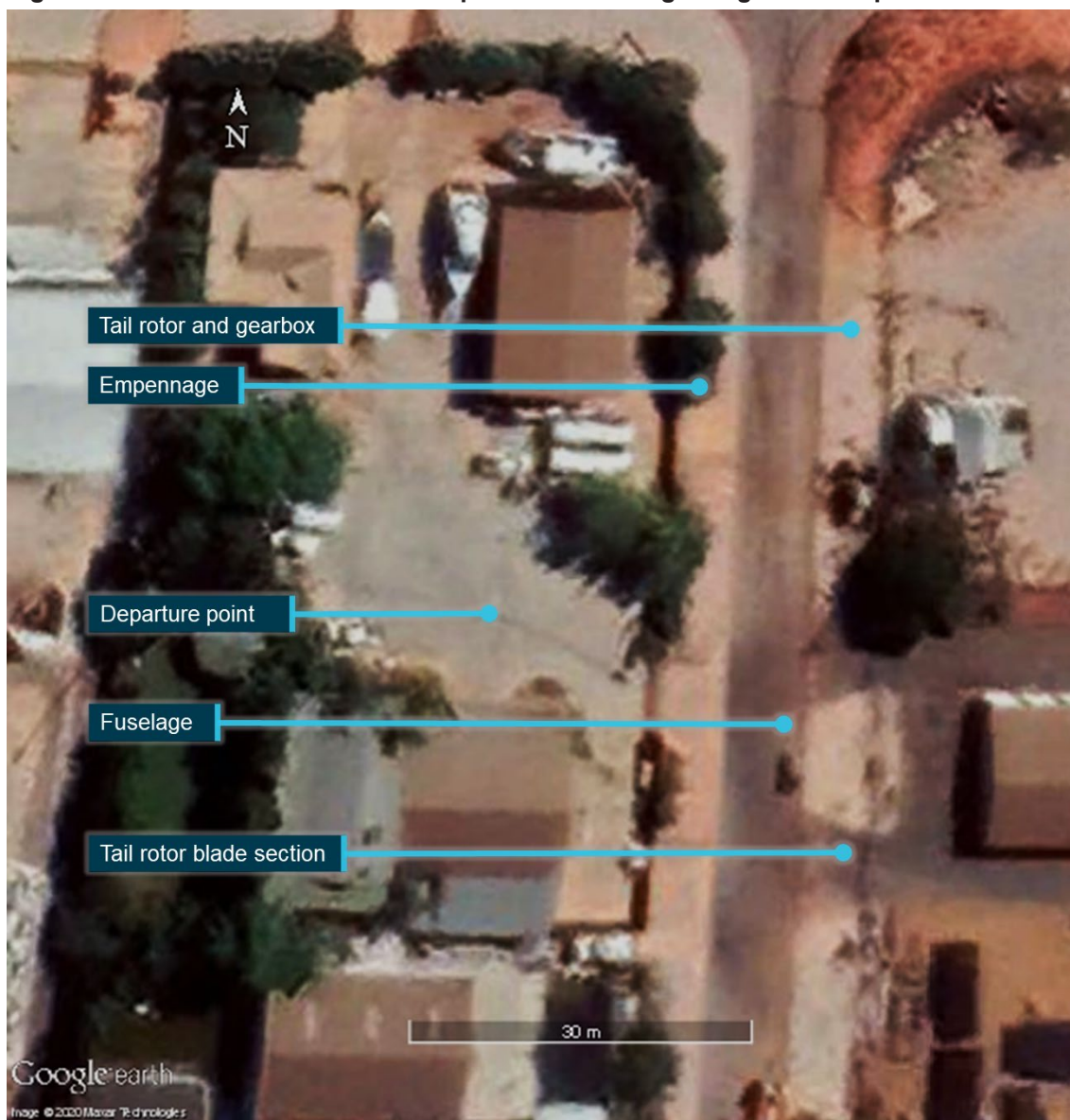
Figure 2: Location of aircraft and components following in-flight break-up
