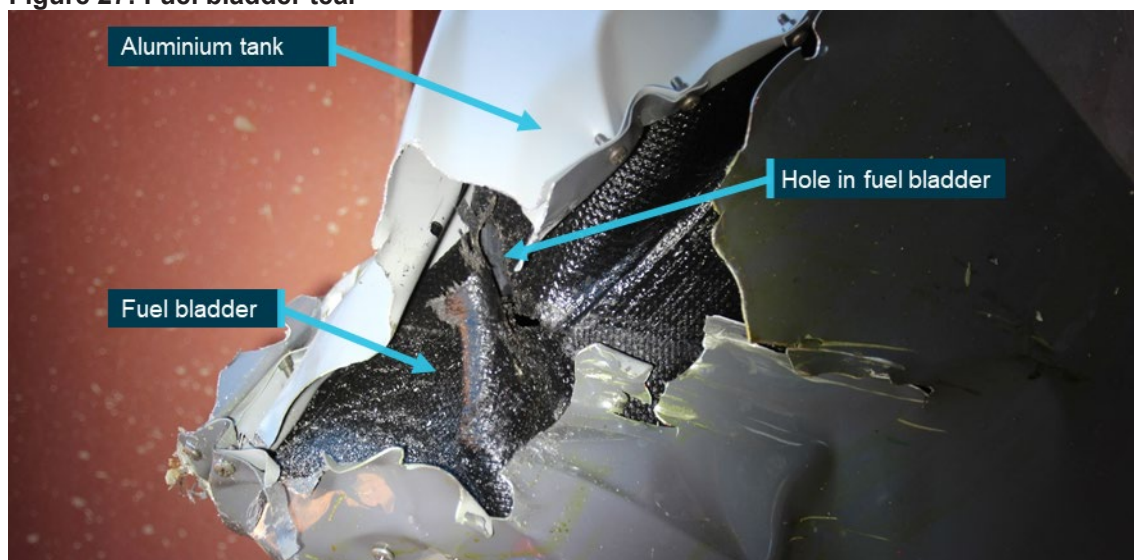
Figure 27: Fuel bladder tear
