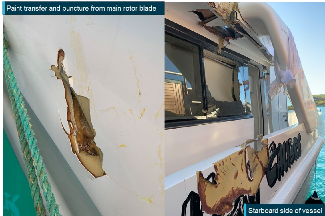
Figure 32: Damage to High Calibre
