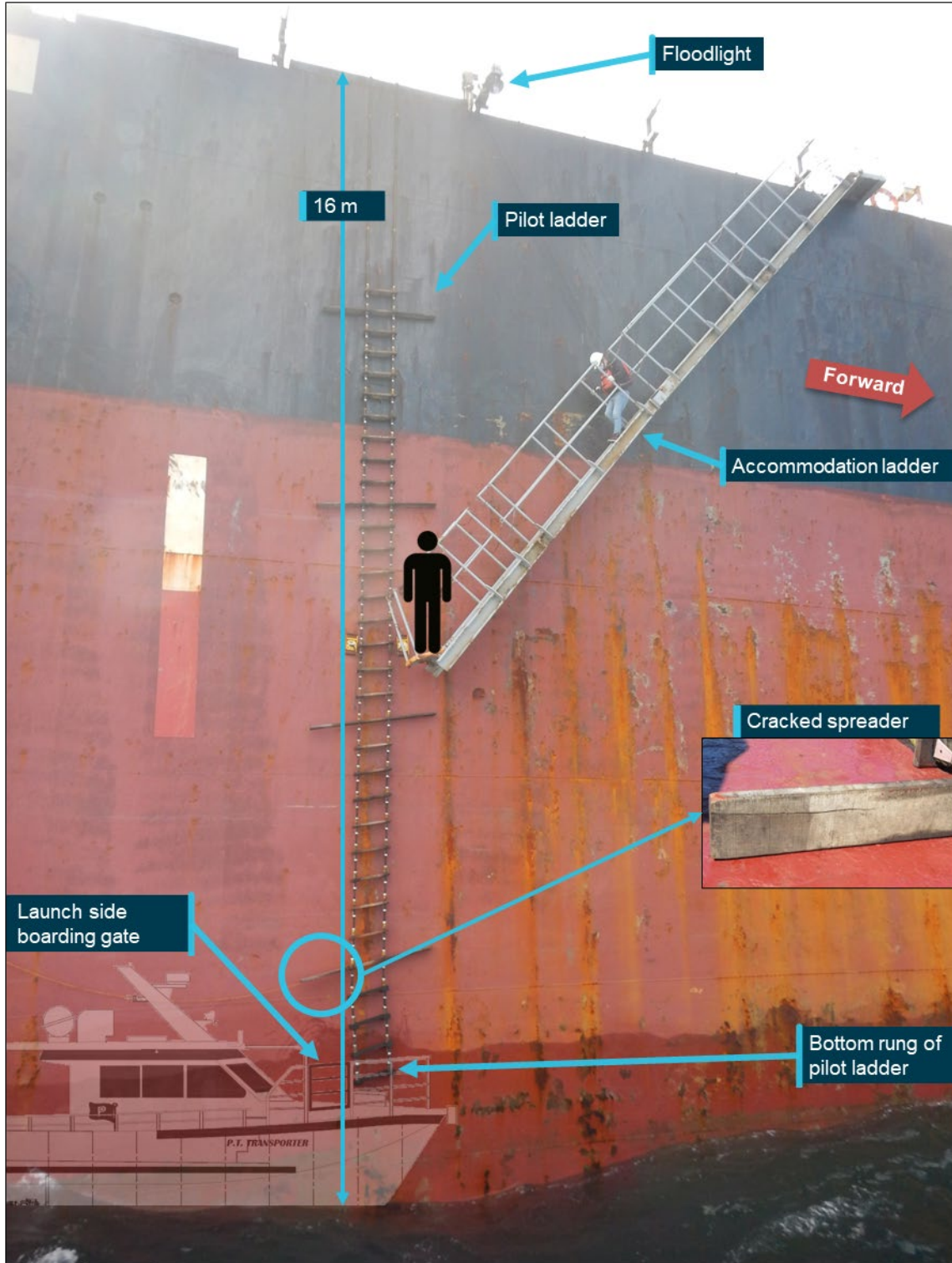
Figure 2: Starboard side boarding site and ladder arrangement
