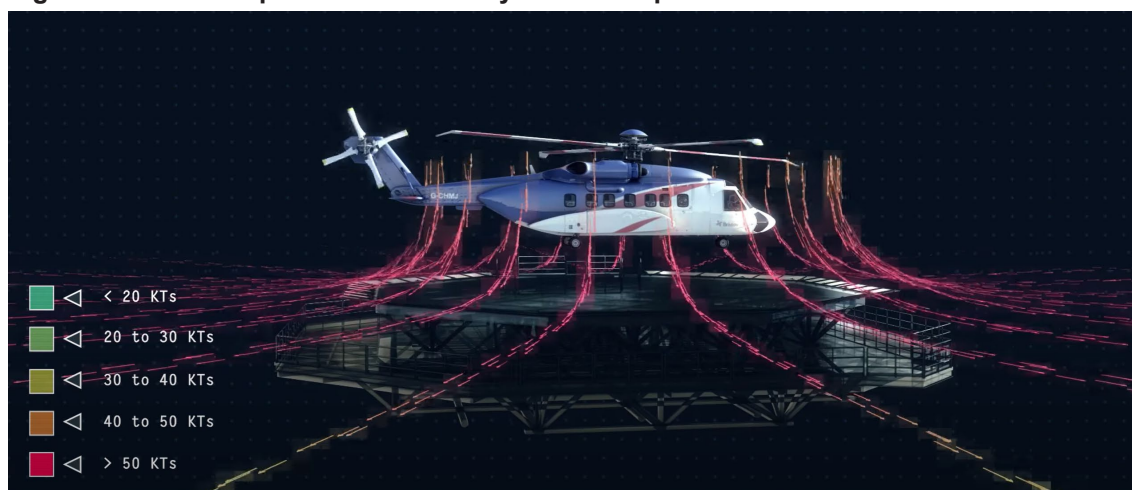
Figure 3: Sidewash profile of a Sikorsky S92 helicopter
