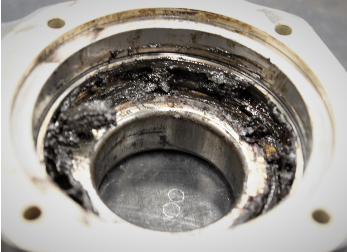
Figure 8: Grease found within the upper bearing
