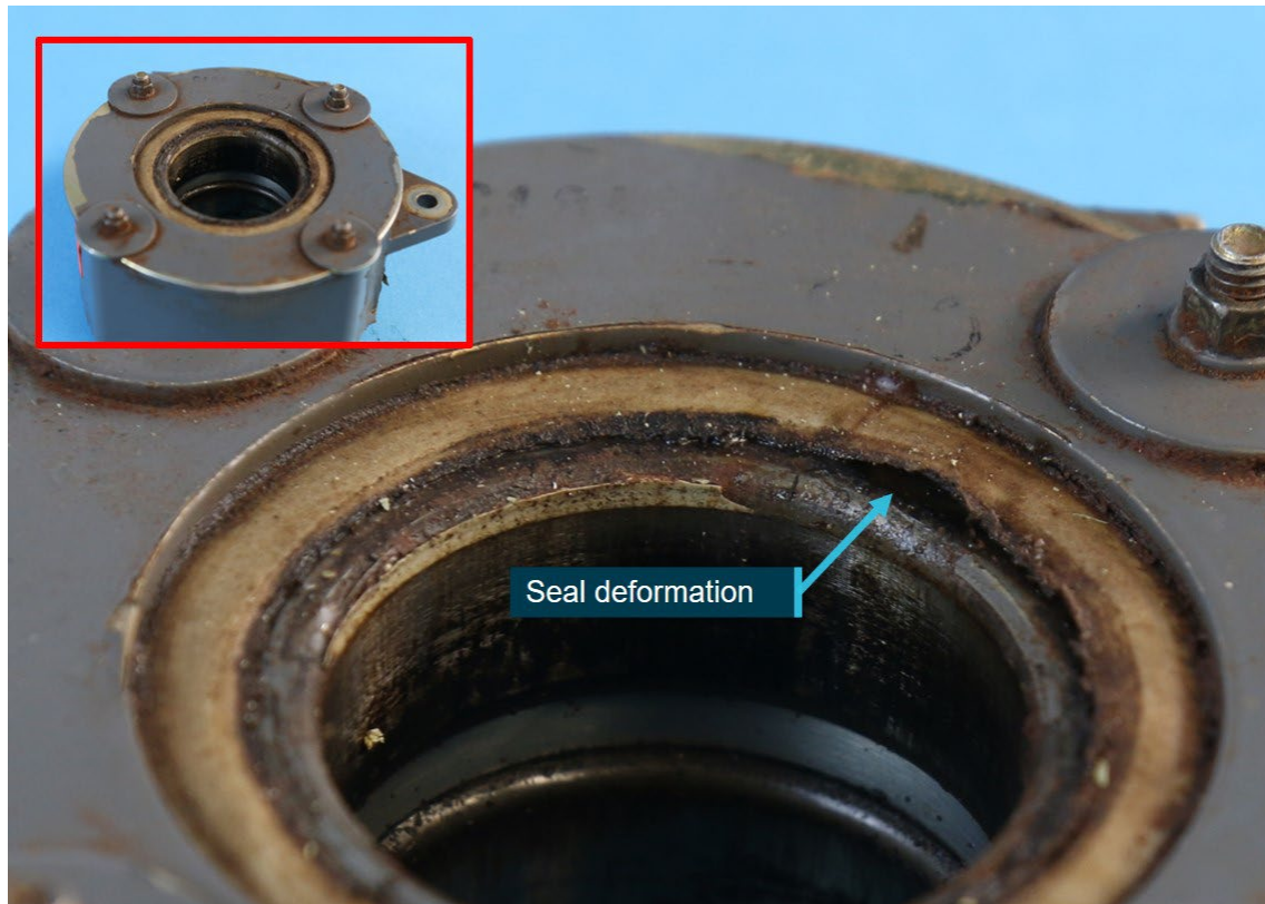
Figure 7: Distortion to the upper bearing seal
