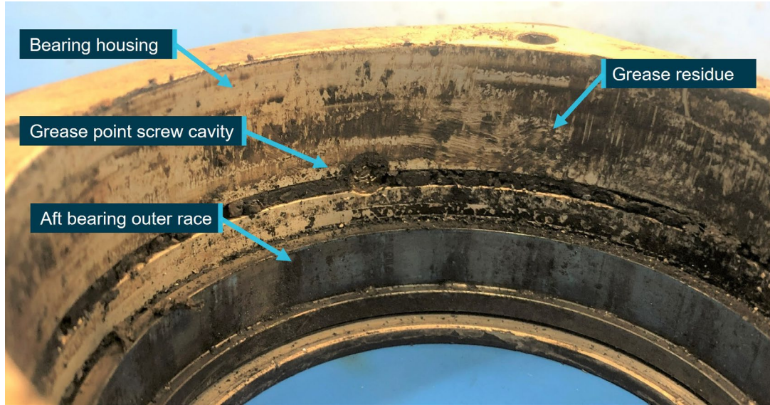
Figure 5: Lower actuator bearing housing, showing minimal dried grease
