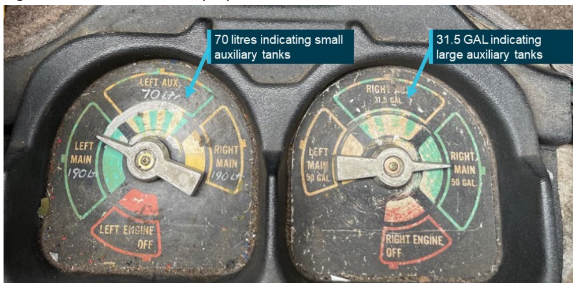
Figure 3: VH-JQK fuel selector plaques
