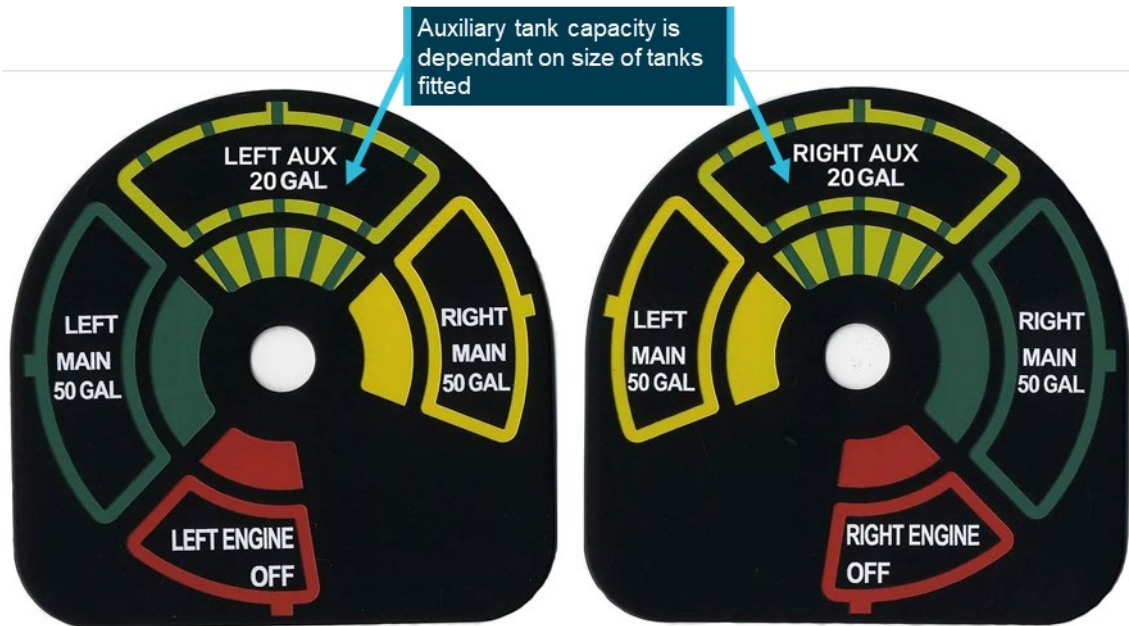
Figure 2: Correct aircraft fuel selector plaques
