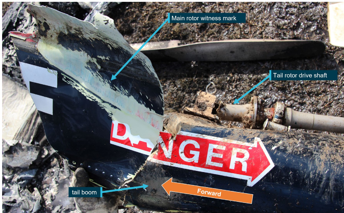
Figure 4: Tail boom impact
