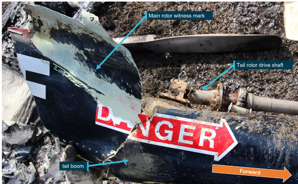
Figure 4: Tail boom impact
